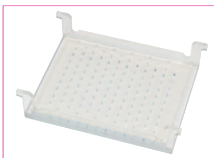
96 format UV tray with a cast gel
